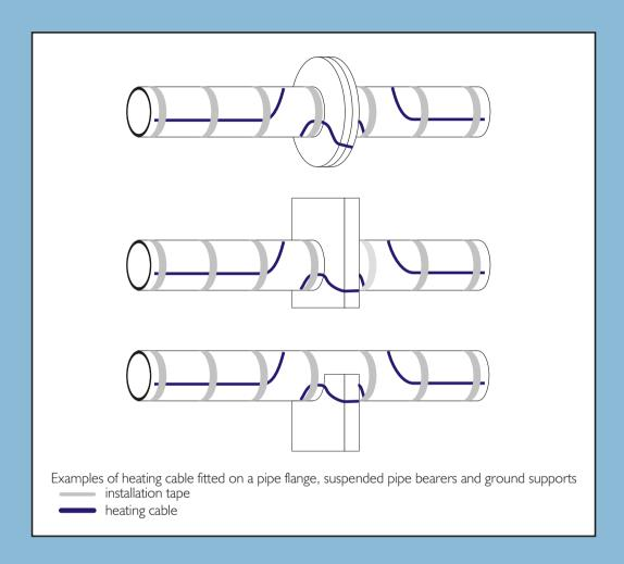
**NOTE:** Heating cables fitted on valves, flanges or supports cannot come into contact with each other. To prevent possible displacement, the cable should be fitted with extra tape lengths.
