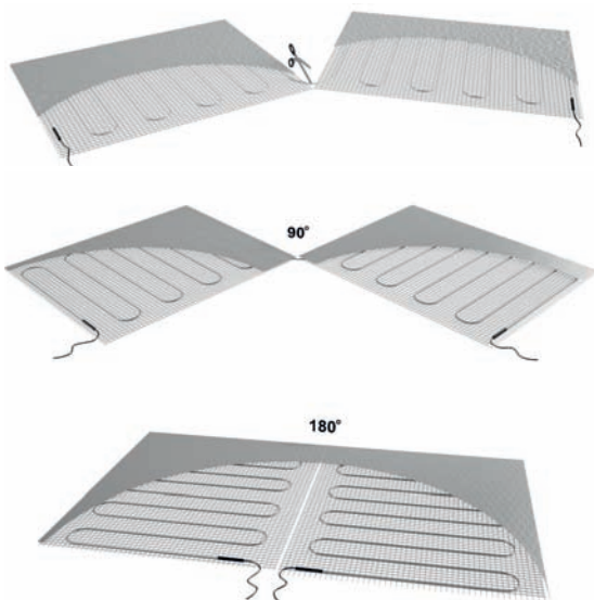
Laying out a custom-shaped heating mat
